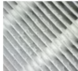
Figure 5. Zeolite coating on the HX
