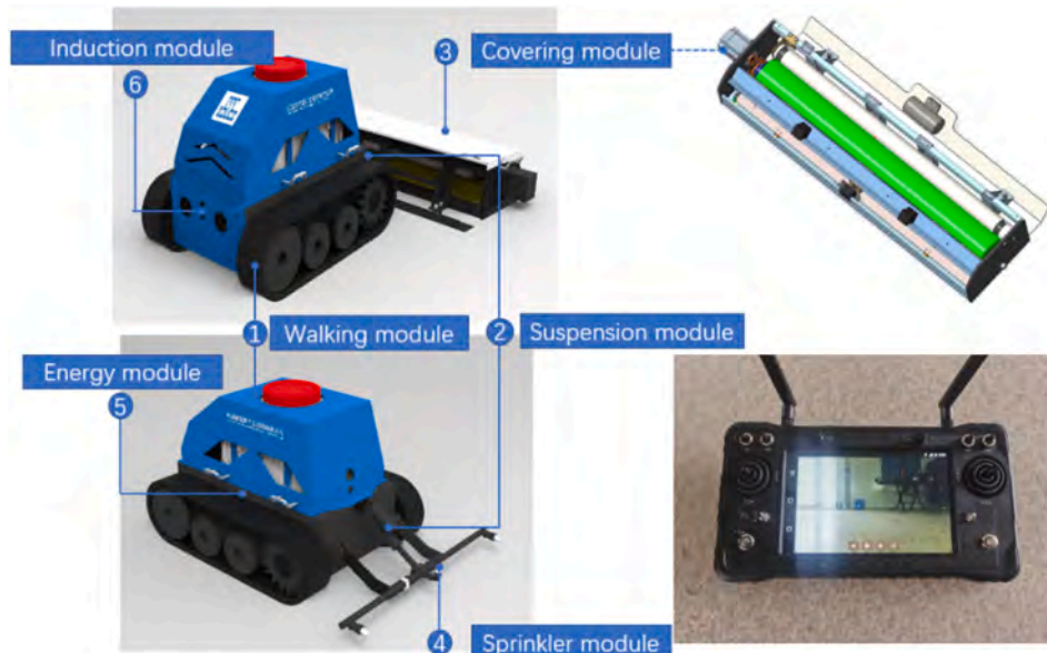
Fig. 2. Structure diagram of the concrete curing robot body and the control terminal.
