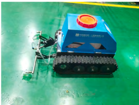
Fig. 6. Robot water spray curing.
