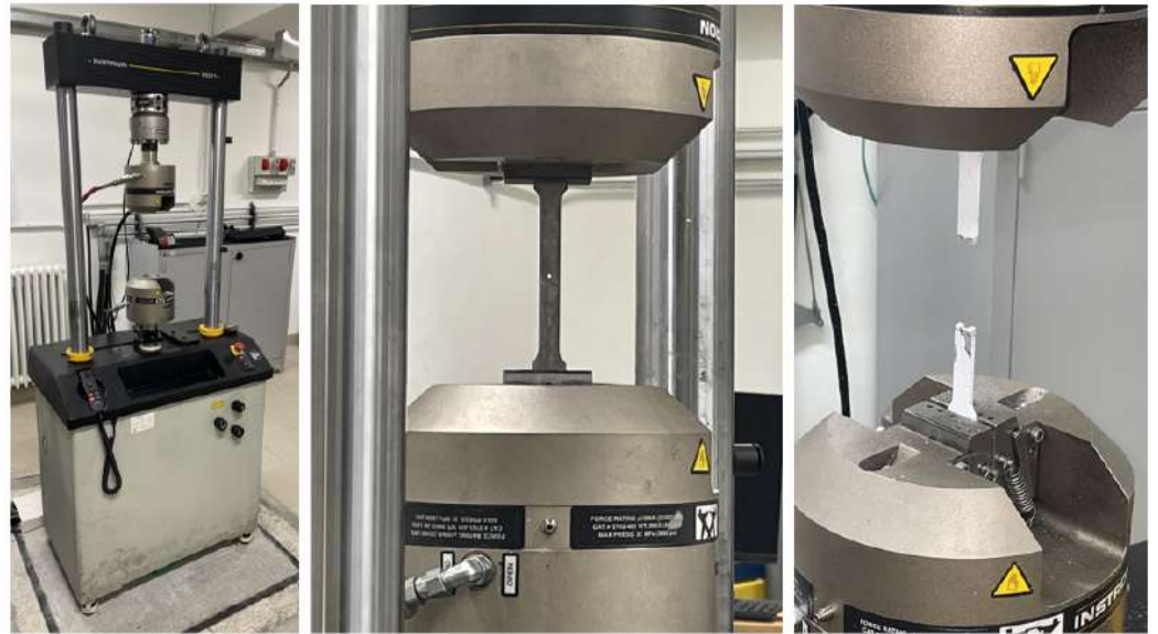
Figure 4. Specimen installed in the fatigue test machine.
