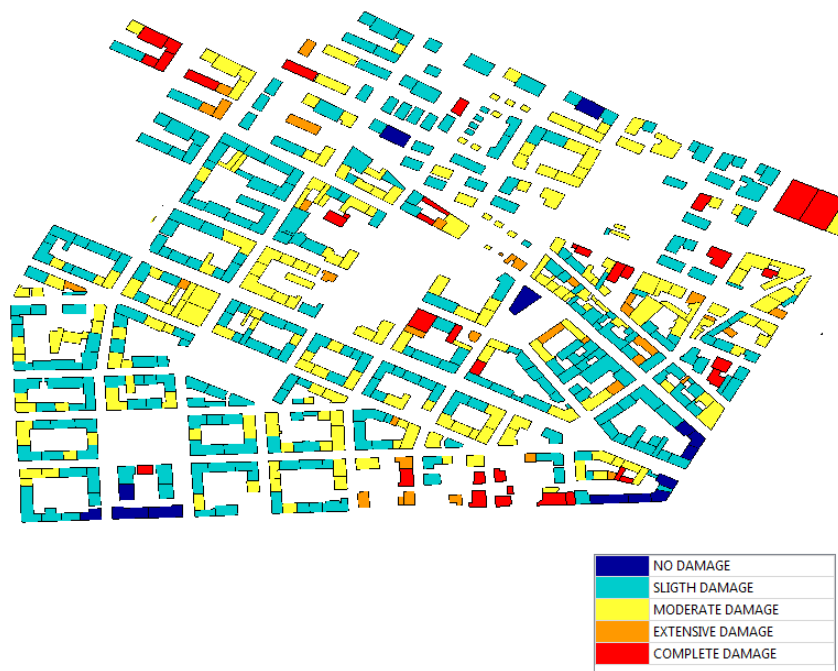
Figure 1. Building damage state.
