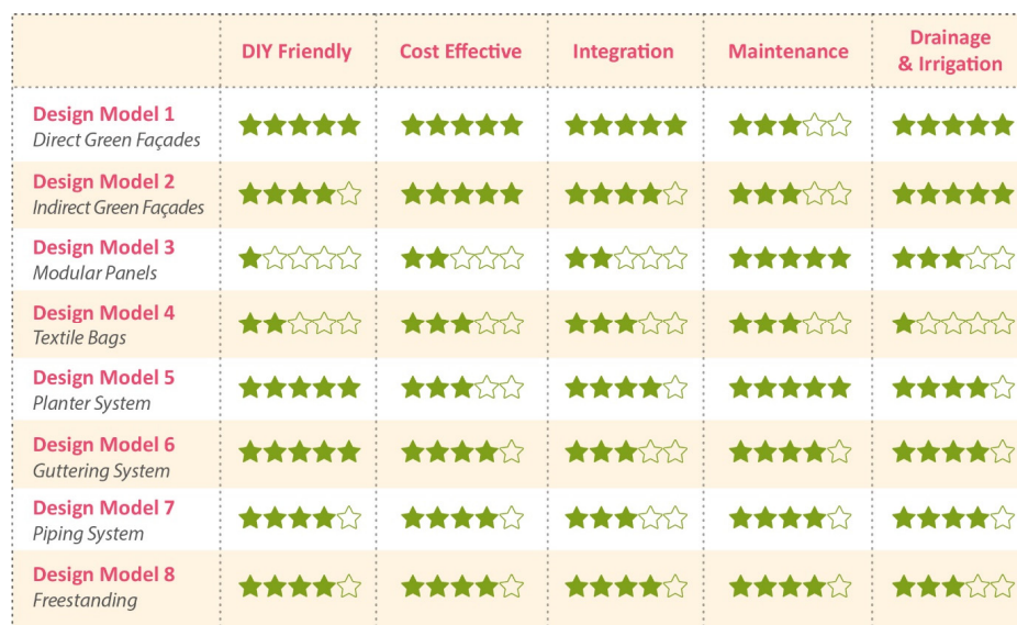
Figure 11. Star-based rating system that compares the VGS designs using community or domestic scale relevant criteria.
