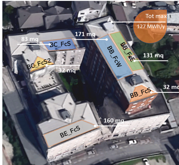
Figure 13: Aerial photo of the condominium subject matter of the case study; colored areas indicate the rooftop selected area described in Table 8
