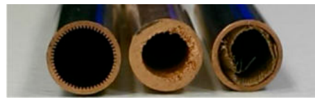
Figure 15. Axial groove, mesh, and sintered cross-section [56].
