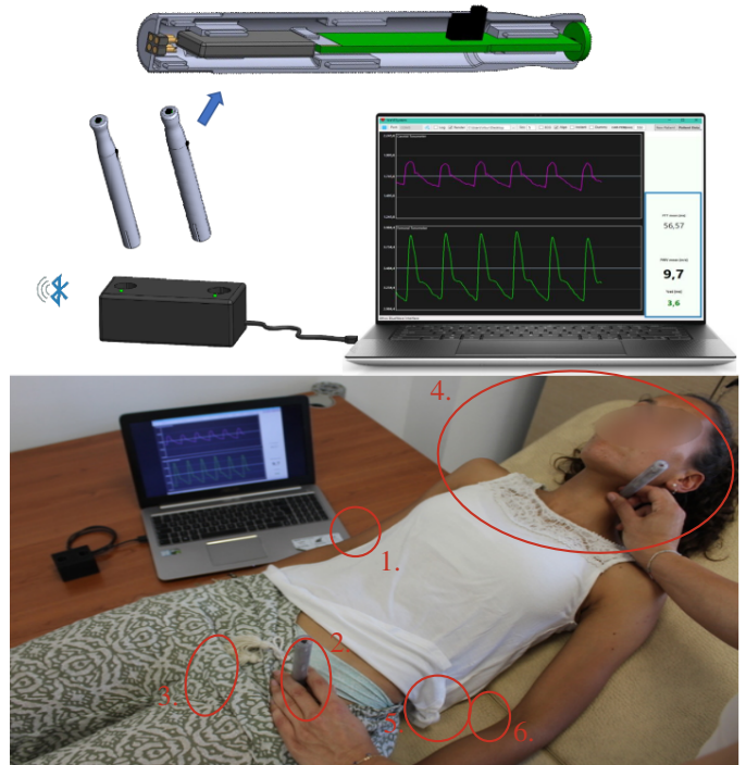
Fig. 1. System setup: 1) Bluetooth receiver; 2) Acquisition device on Extensor Carpi Ulnaris ; 3) Acquisition device on Palmaris Longus ; 4) System GUI while plotting ATC values; 5) Employed electrodes; 6) Involved PCB.
