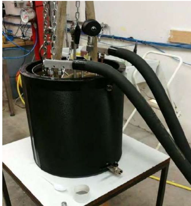
Figure 2. Reactor in the thermostatic bath.
