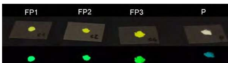
Figure 1. P and FP samples in their inactive (above) and active (below) state.
