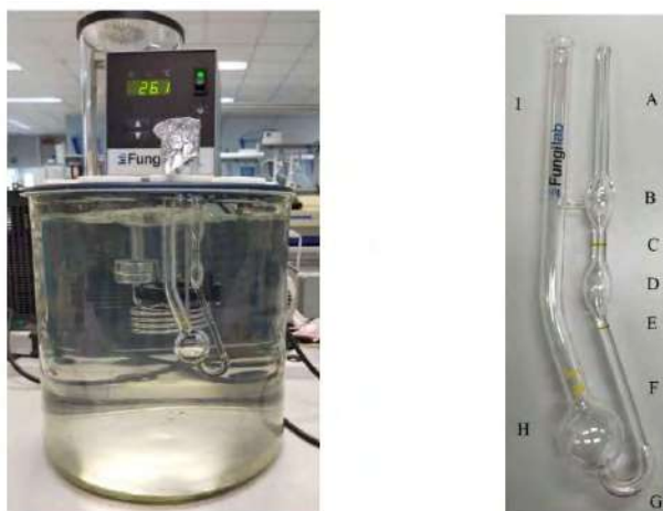
Figure 2. Experimental setup and viscometer.
