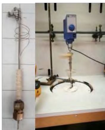
Figure 1: High-pressure batch reactor assembly
