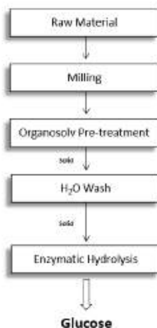
Figure 1: Flowchart of the organosolv pre-treatment process
