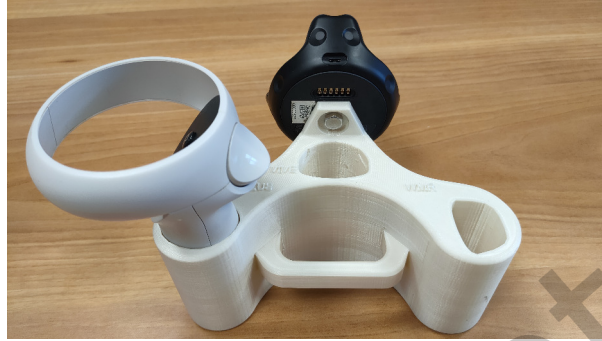
Fig. 2. 3D printed prop used for calibrating the Meta Quest 2 and HTC Vive reference systems.
