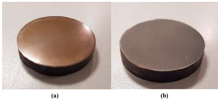
Fig. 2 a) Surface polished with 600 \mu\text{m} sandpaper b) Raw surface after EDM processing
