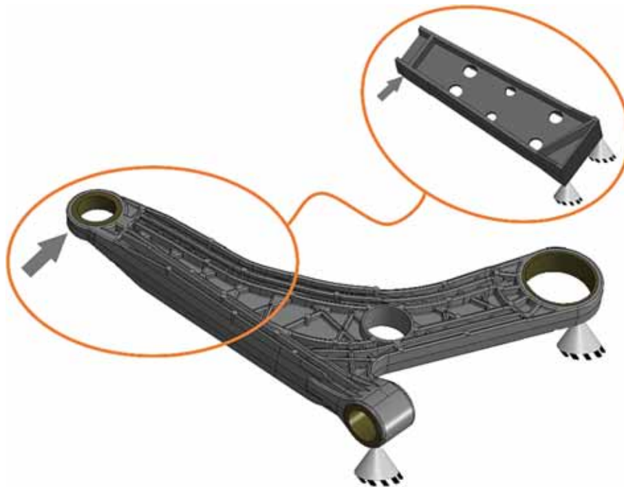
Fig. 1. Geometry simplification from the real suspension arm to the analysed demonstrator. Loading conditions of the control arm are also reported.
