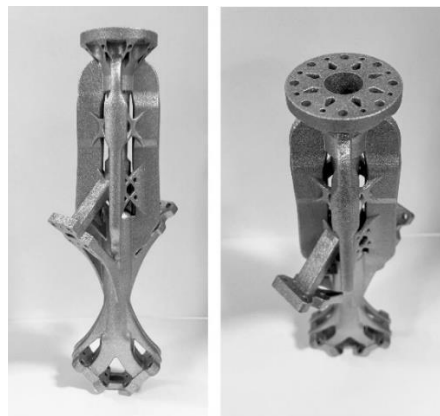
27 28 29 30 31 32 33 34 35 36 37 38 39 40 41 Fig. 1 Example of an RF component: a monolithic K/Ka-Band Dual-Circular Polarization Antenna- 42 Feeding Network [22]. 43
