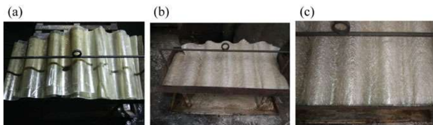
Fig. 5 a Waste Ref. A2 in Solvo Line oven tray, b Obtained product, c Clean rGF with mat format
