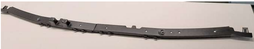
Fig. 16 Prototype cowl top support with rGF
