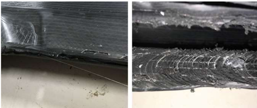
Fig. 4 Disassembly procedure for adhesive joints using the wire saw technology, cutting process (left) and cutting edge after separation (right)
