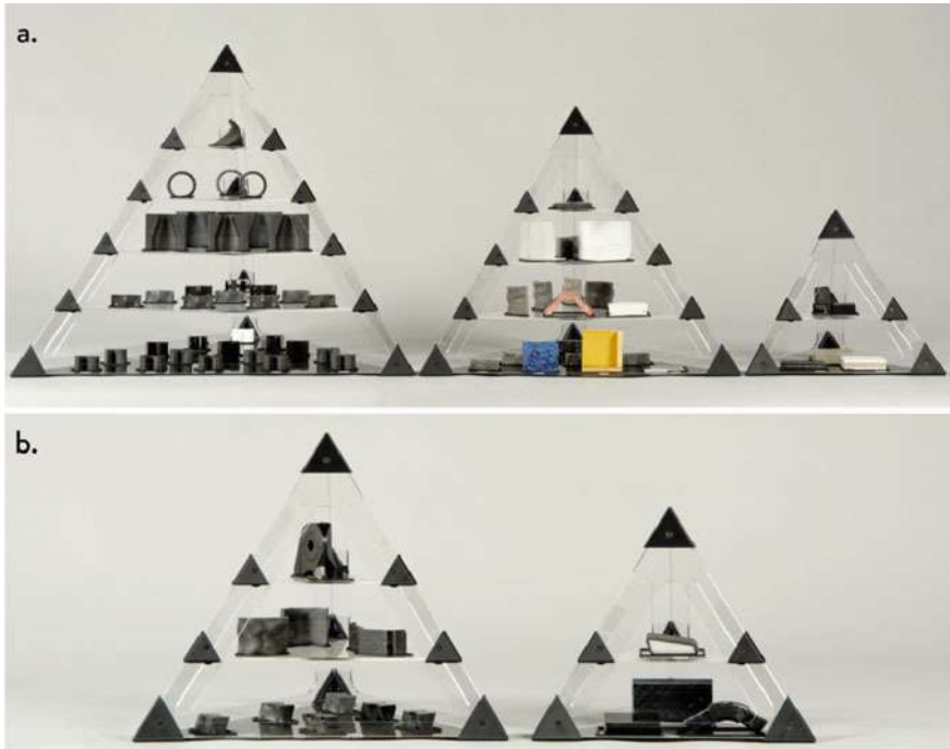
Fig. 6 Physical Product Library: a GF structures (from left to right: “liquid deposition modelling—3D printing, casting, lamination and injection molding”); and b CF structures (from left to right: casting and injection molding, reuse of components)
