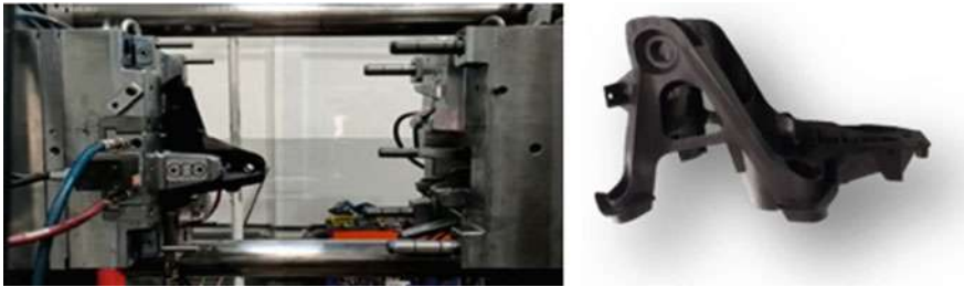
Fig. 6 Pedal mould (left) and prototype manufactured with PARCF20 (right)
