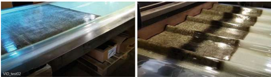
Fig. 19 rGF Mat processing
