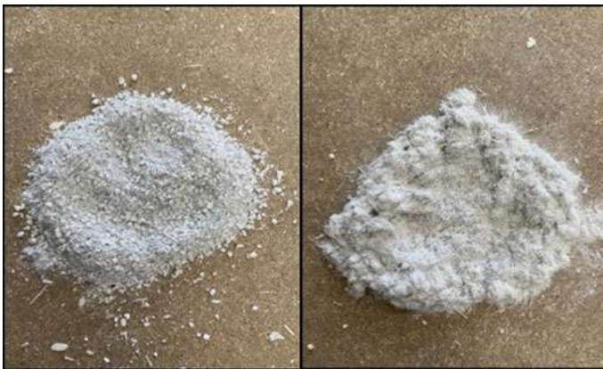
Fig. 2 Different types and sizes of mechanical recycled granules from shower trays windblades and GFRP roofs (< 2 mm particle size above, > 2 mm below)
