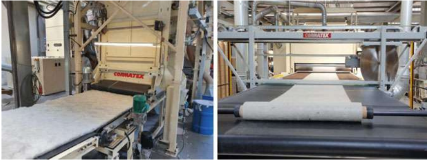
Fig. 17 Cormatex industrial production of rGF mat
