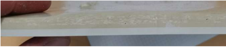
Fig. 5 Cross section of shower tray with rGFRP
