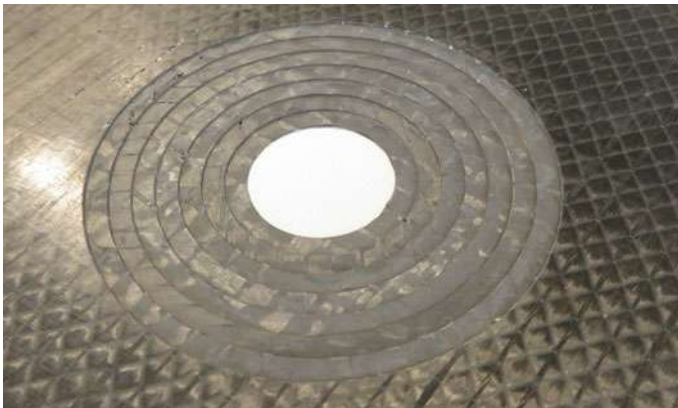
Fig. 2 Removed defect caused by an impact
