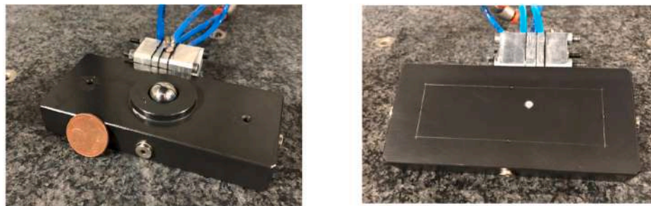
a: Prototype of air pad compensated by a differential diaphragm valve.
