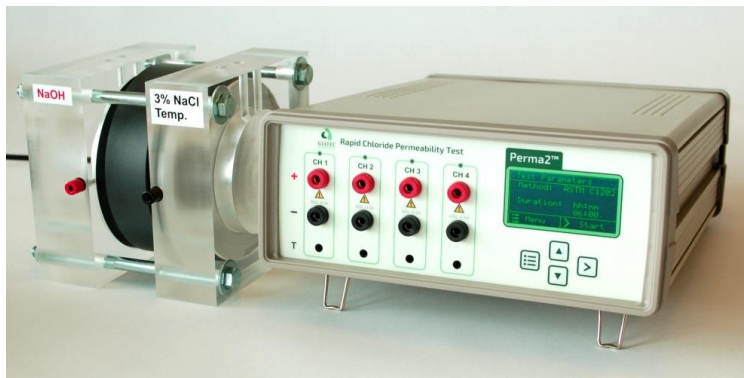
Figure 9. Test cell and Perma 2™ voltage applicator.
