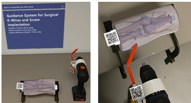
Figure 9: Guided K-wire Insertion in a Dummy: Virtual Overlay Revealing Internal Structures with the K-wire Tip Indicated by a Red Cylinder. Tracking achieved via QR code mounted on the drill, utilizing Vuforia™Instance.
