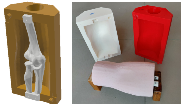
Figure 6: Left: rendering of humerus, radio and ulna with negative soft tissues mold (side B); Right: physical phantom on wooden supports and molds (from left to right: side A and B)
