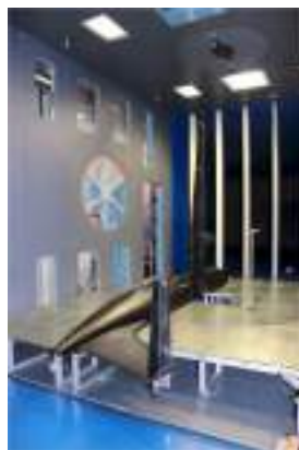
Figure 2: Photo of the aeroelastic half model installed on the WAS system (left) and the gust generator (right)
