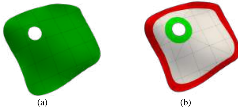
Figure 1 Same shell structure discretized using a trimmed single patch (a) and a combination of a main patch and two auxiliary boundary conformal ones (b).
