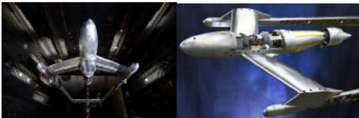
Figure 3: SUBLIME BLI360 configuration in wind tunnel
