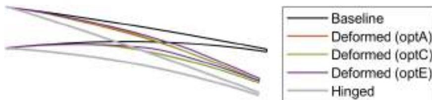
Figure 2: Morphing shapes and hinged shape corresponding to target C_L=1.15 .
