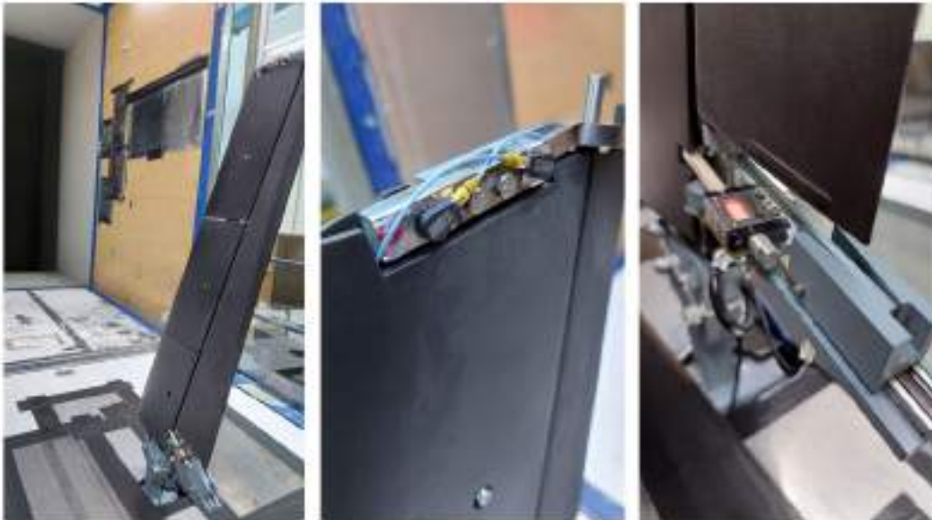
Figure 1: Photo of the test model, installed in the wind tunnel
