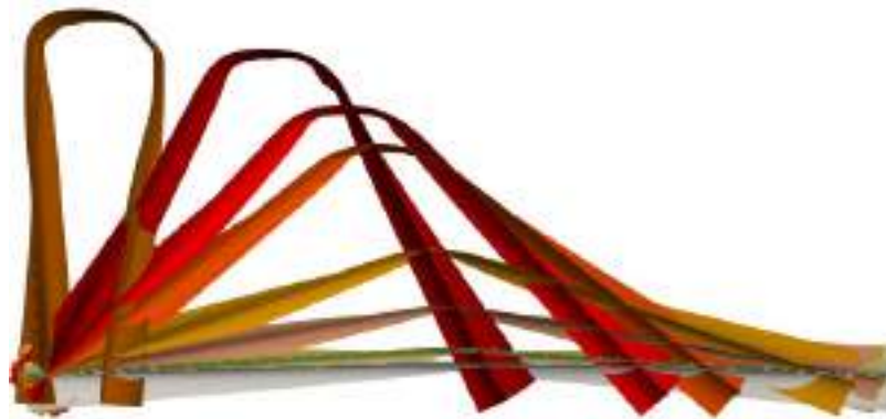
Figure 7 - Folding simulation of the TRAC longeron without contact mechanics
