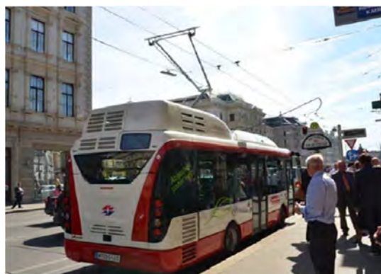
Figure 14. Siemens-Rampini two-pole pantograph for contact with the overhead line.
