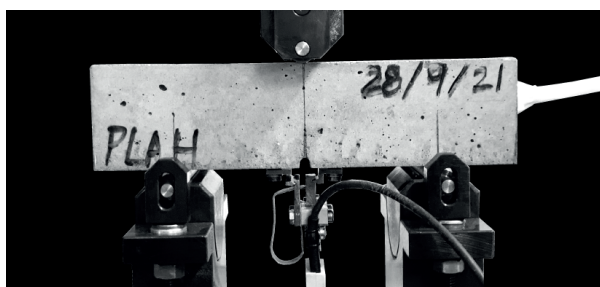
Fig. 3. Sample during the pre-cracking step; on the right side, the tube for the water flow test is visible.
