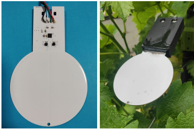
(a) Prototype of the LWS (b) LWS on the field Fig. 3. Final LWS prototypes
