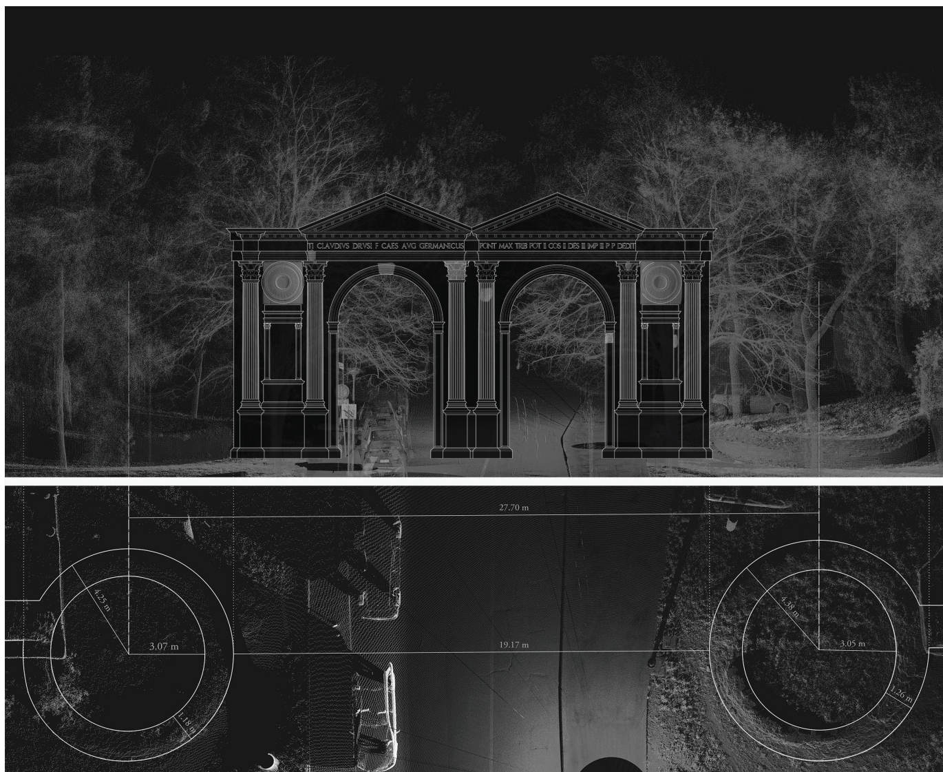
Fig. 13_ Point cloud obtained from laser scanning acquisition. Plan view with dimensions. The Roman Gate was framed by two round towers (bottom). Front view of evidences of the towers with superimposition of hypothetical virtual reconstruction based on A. Palladio drawings and dimensioned using photogrammetric acquisition of fragments conserved in the Museum (top). Image by the Author.
