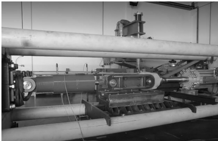
Figure 2: FVD specimen on the test facility at SISMALAB
