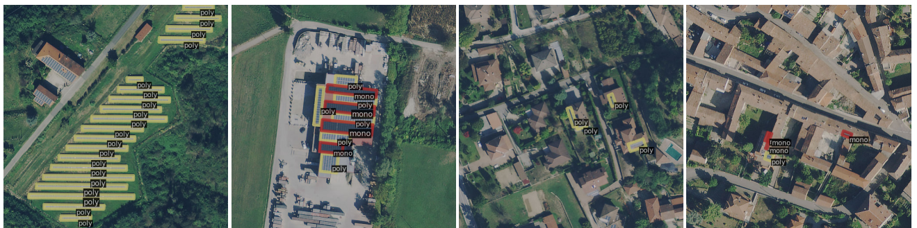
FIGURE 2. Examples tiles extracted from the dataset, together with their annotations. Starting from the left, the first two images show large industrial installations, employing both monocrystalline and polycrystalline panels, while the last two illustrate the smaller domestic installations.
