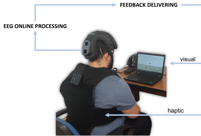
Figure 1. A subject using the proposed BCI system with neurofeedback in extended reality. The system involves EEG acquisition with the Helmate device, online processing, and actuators for visual-haptic feedback delivering.
