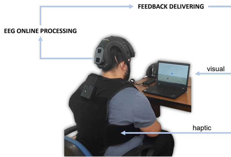
Figure 1. A subject using the proposed BCI system with neurofeedback in extended reality. The system involves EEG acquisition with the Helmata device, online processing, and actuators for visual-haptic feedback delivering.
