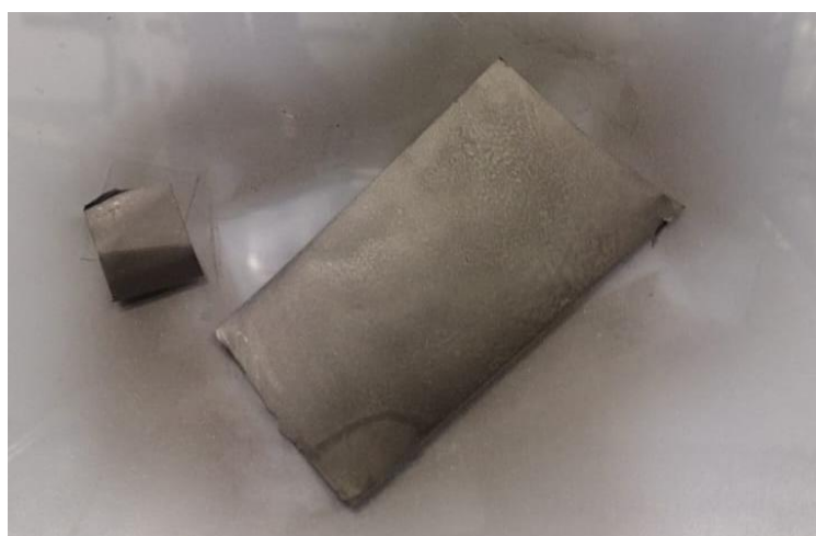
Figure 24 PSU coated with GEM using the airbrush.
