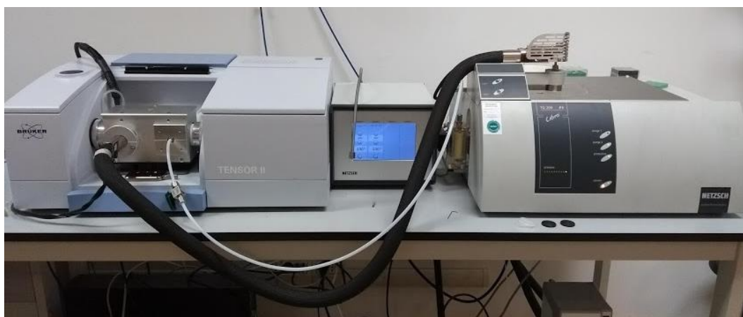
Figure 26: Thermo-gravimetric analyzer coupled with infrared spectrometer a Right: TGA instrument; left: IR spectrometer equipped connection for gas-phase transmission of decomposition products; center: heated transfer line and temperature controller.
