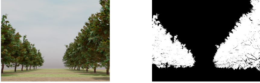
Figure 3.2: An example of synthetic RGB image obtained in a simulated row-based field and the corresponding segmentation mask.
