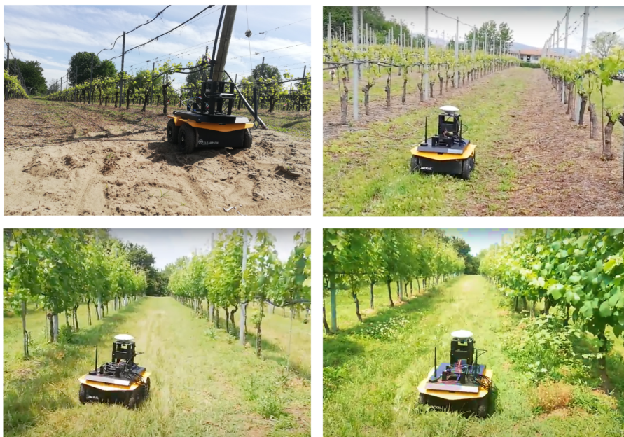
Figure 1.1: The Clearpath Robotics Jackal UGV while autonomously navigating in an agricultural environment
