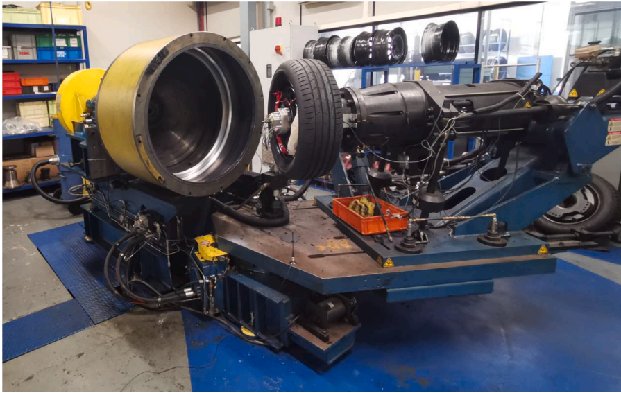
Fig. 10. MTS 855 wheel biaxial fatigue test bench (courtesy of MW Italia S.r.l.).
