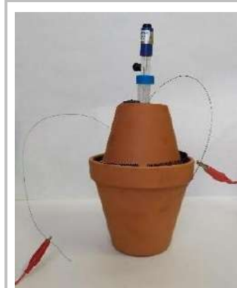
Figure 13 - Lab-scale bio-electrochemical power-to-methane
