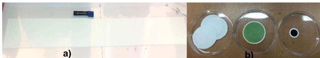
Fig. 1. Photographs of (a) the top view of the green tape and (b) sintered cells.
