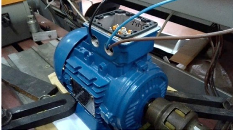
Fig. 2. The 550W TENV induction motor.
