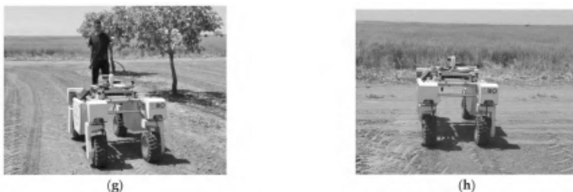
Figure 9. Snapshots from experimental demonstration session in an orchard depicting (a) the locking onto of the first person by the UGV, as well as the UGV (b) following the locked participant, (c) stopping, and (d) unlocking this participant. Next, the UGV (e) locked onto the second participant, (f) followed him, (g) was ordered to go to the target location, and (h) reached this location.
