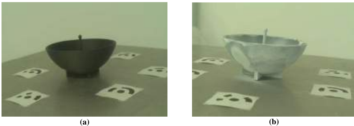
Figure 3 Representation of the component without surface treatment (a) and covered with a solvent-based anti-reflex spray (b).
