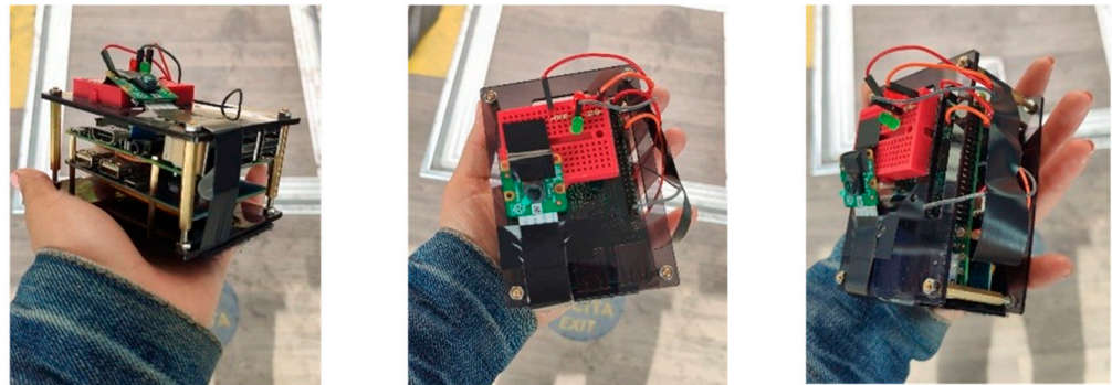
Figure 2. Low-cost APC system.
