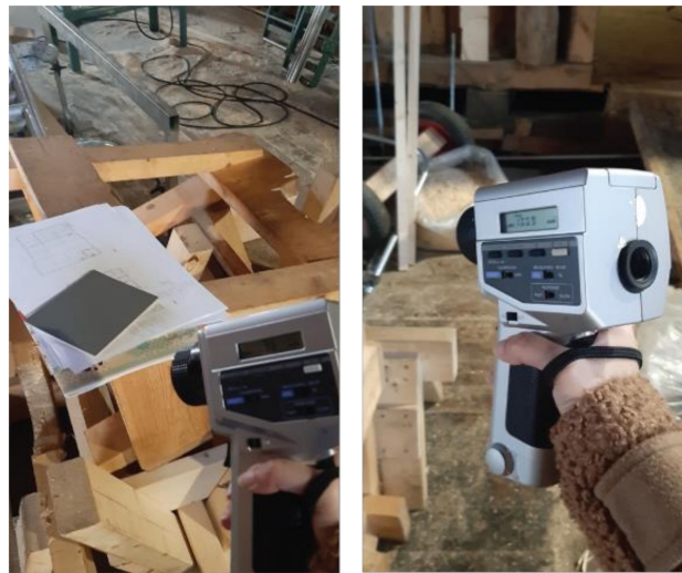
Figure 5. Field luminance measurement is used to calculate the light reflectance of real materials for simulations [44].
