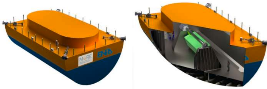
Fig. 2. Render of the PEWEC hull, the Pendulum and the PTO.
