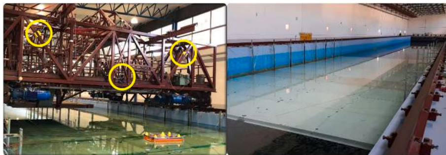
Fig. 9. Qualisys cameras position and shoal artificial seabed.
