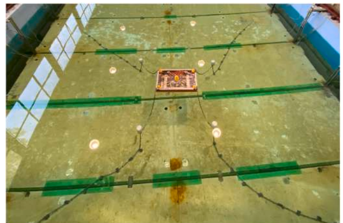
Fig. 3. PEWEC Mooring system 1:25 scaled model.
