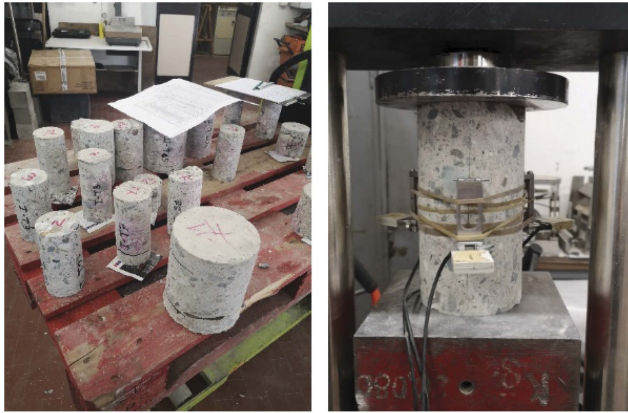
Figure 7. Uni-axial concrete compressive test for elastic modulus assessment.
