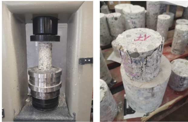
Figure 5. Uni-axial compressive strength tests on concrete samples.
