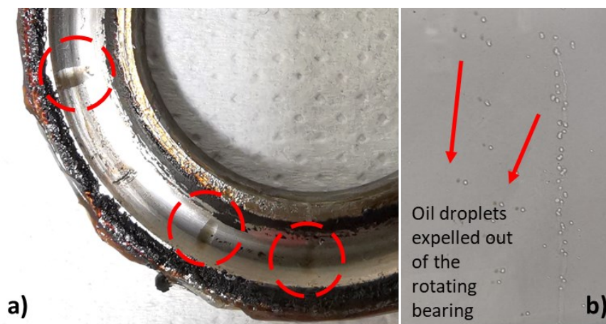
Figure 156: (a) Grease base oil drained from the spheres in static contact over the ring after the end of a test (Test 3); (b) Oil droplets expelled out of the DUT and accumulated on the safety enclosure of the test rig.
