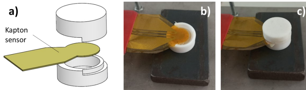
Figure 90. (a) Special grease box for Hot Disk test on graphene-grease compound; (b) experimental setup of the tests.
