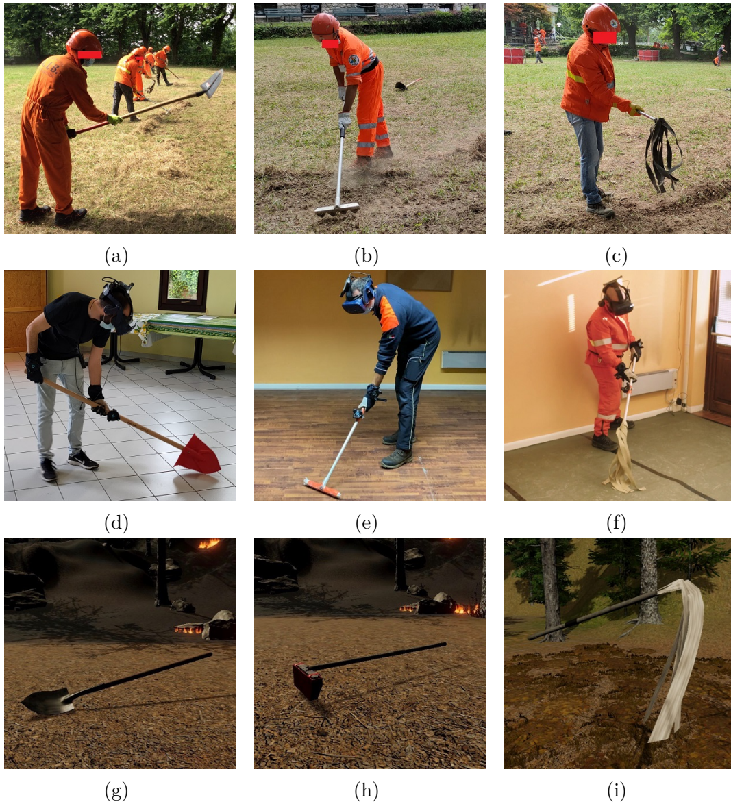
Figure 2.10: Considered firefighting equipment (shovel, McLeod, and broom): real usage (a–c), PH props (d–f), and virtual replicas (g–i).
