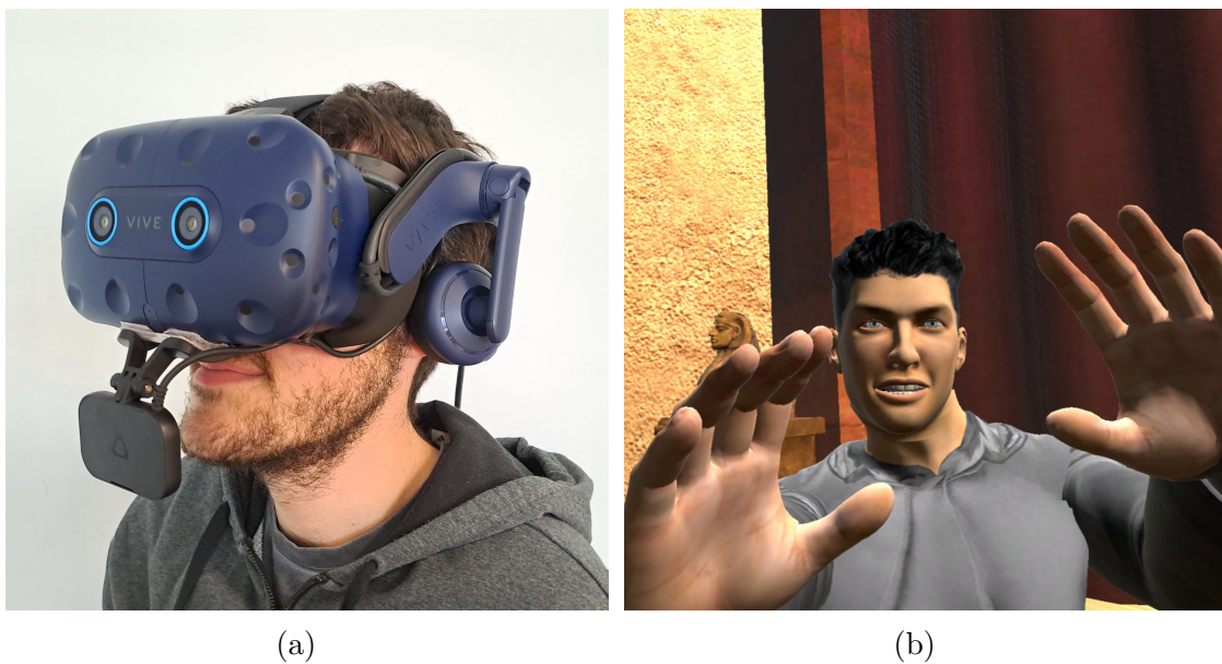
Figure 3.12: VR setup selected for the experimental activity (HTC VIVE Pro Eye + Facial Tracker) (a). Close-up of the user’s avatar (b).
