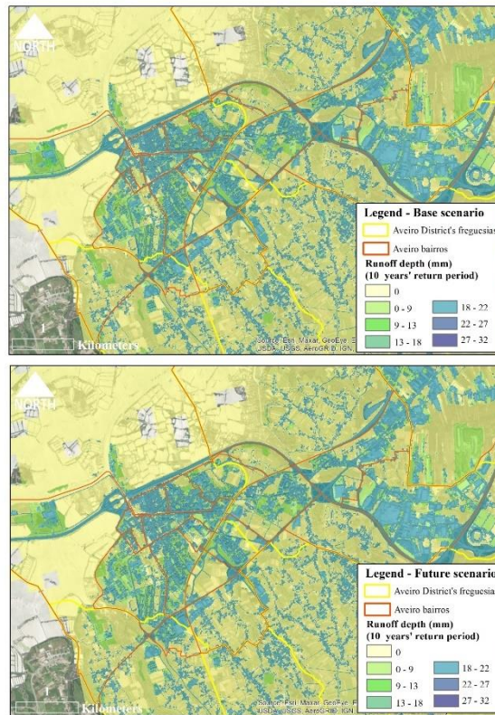
Figure 68. Flood depth (mm) under 10-year return period per pixel for current & future scenarios (city of Aveiro).
