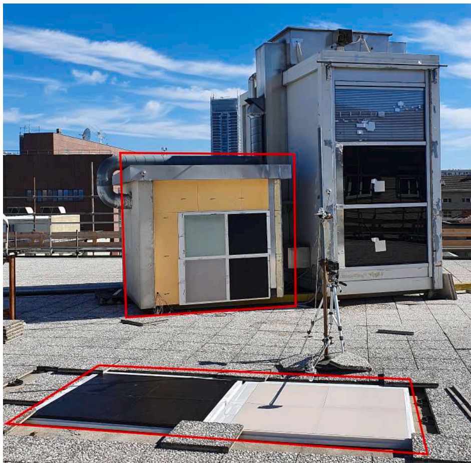
Fig. 3. Picture of the outdoor test facility with the experimental set-up highlighted in red; the picture was taken on the first day of experimentation.
