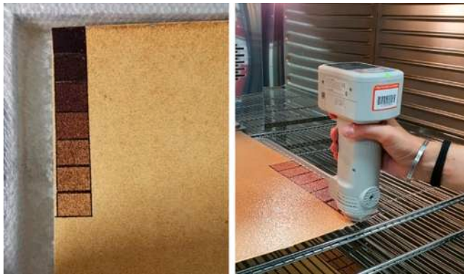
Fig. 6. Pictures of the two testing conditions for the measurements used to assess the unexposed panels and the photodegradation of the exposed ones (shown in the pictures), i.e., a) the ice basin, b) the ventilated oven.
