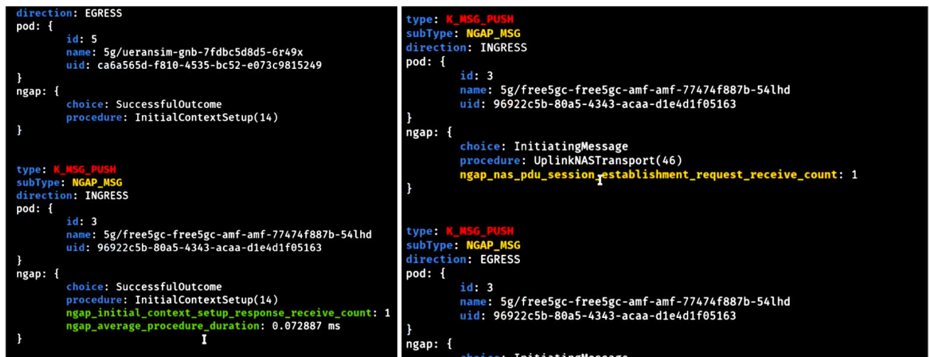
FIGURE 28. Examples of 5G gauges and counters derived by the Sauron Agent (daemonset) in real time.
