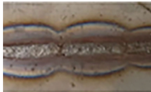
Fig. 19 SMAW bead surface
