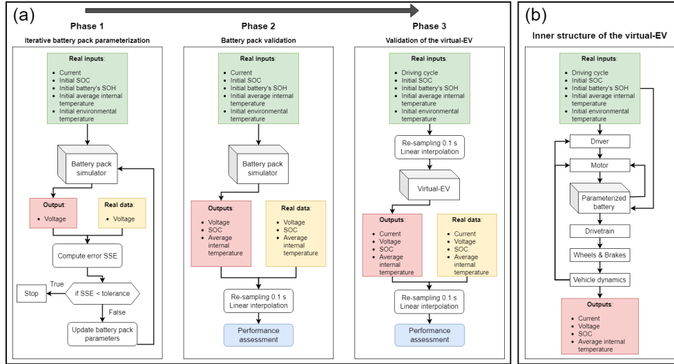
Fig. 1. (a) The complete pipeline of the proposed methodology, which starts with the battery pack parameterization (phase 1), followed by the validation of the tuned battery alone (phase 2), and, lastly, the validation of the full virtual-EV (phase 3). (b) The inner structure of the virtual-EV.
