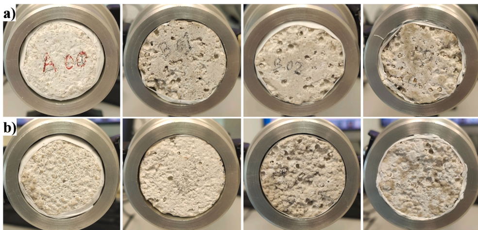
Fig. 5. The A00, B01, B02, and B03 samples inside the Impedance tube. a) front and b) back of each sample.
