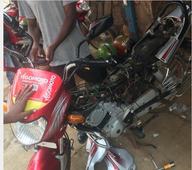
Figure 17: Installation of a YegoMoto ICFM (© Sebarenzi Alexis)
