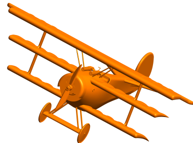
Fig. 9. Model of a Fokker Dr.I with an approximate wingspan of 7 m. The model is discretized with 196 280 triangles and 294 420 RWGs.
