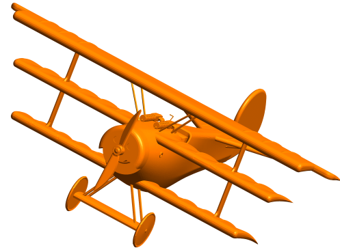
Fig. 12. Model of a Fokker Dr.I with an approximate wingspan of 7 m containing N_H = 390 global loops. The model is discretized with 196 280 triangles and 294 420 RWGs.
