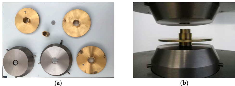
Figure 12. The specific cylinder with dedicated tools: brass cylinder and separator discs with dedicated extension poles (a); insert in hysteresisgraph joke (b).
