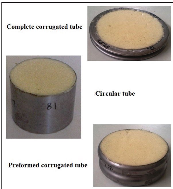
Figure 2. Foam-filled steel E304 tubes of three different geometrical types before the tests.
